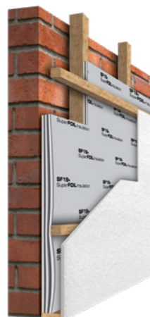
Diagram 2 - Typical detail of System installation with battens and plasterboard
